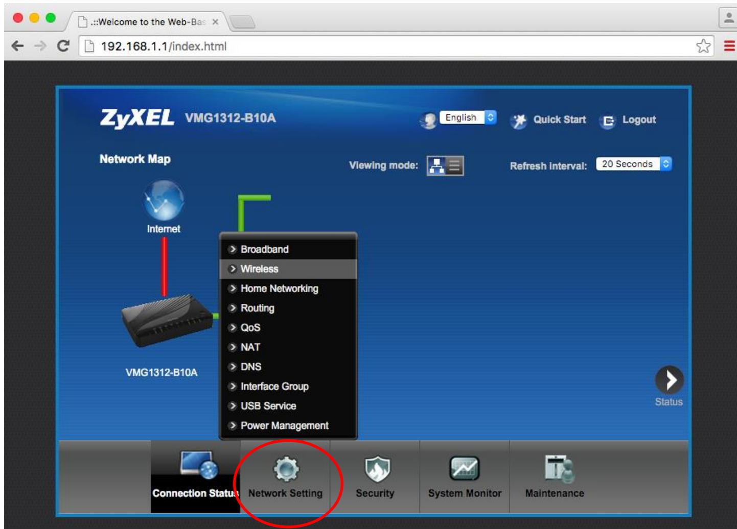
Once in the wireless section of the router you will see "Wireless Network Name (SSID)" below the heading "Wireless Network Settings". Change the value in this box to change the SSID. Here you can also choose whether to broadcast the SSID or not, set the maximum number of devices allowed to connect wirelessly, and the maximum download/upload bandwidth allowed for wireless traffic.
